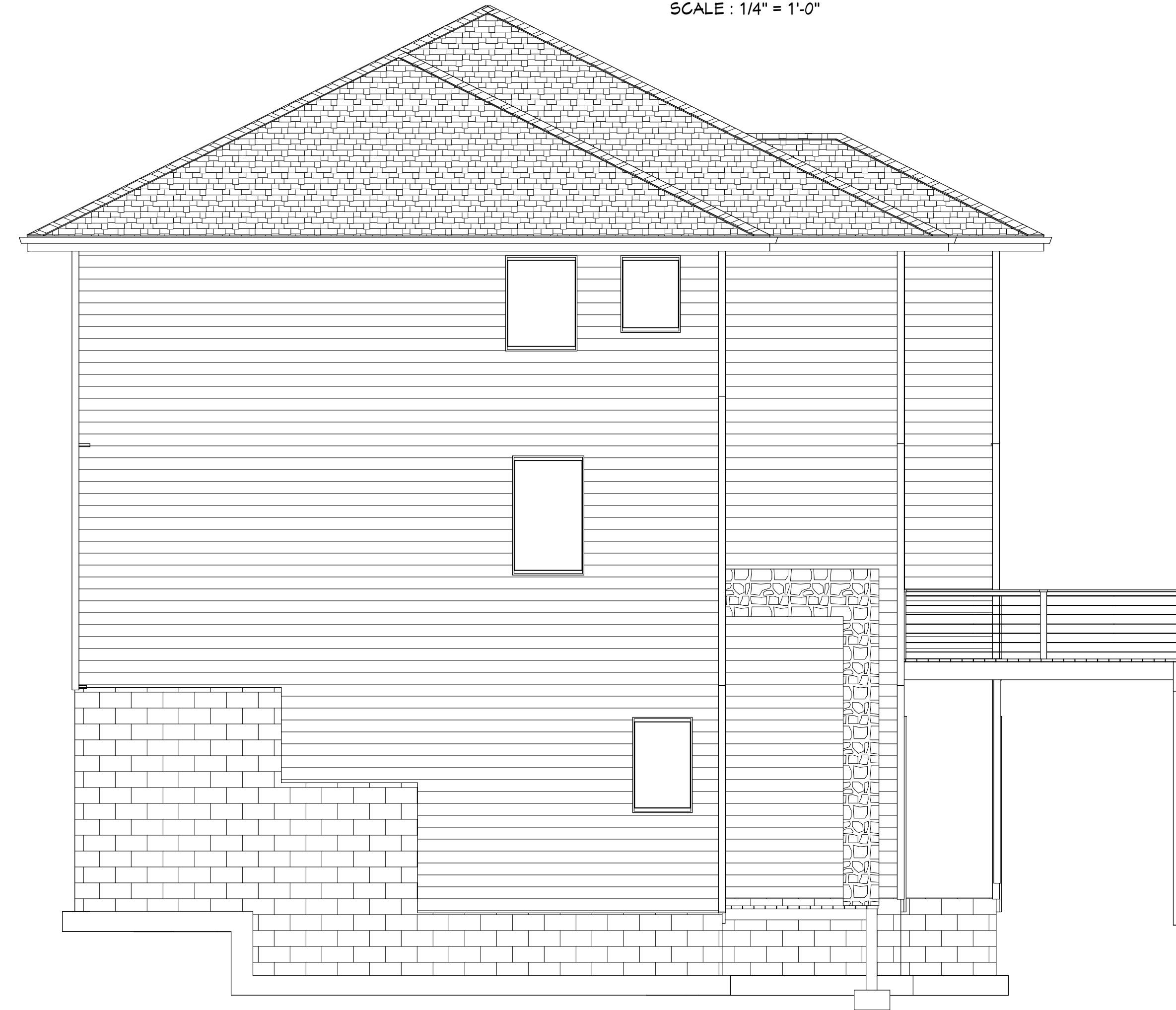
LEFT ELEVATION SCALE : 1/4" = 1'-0"
