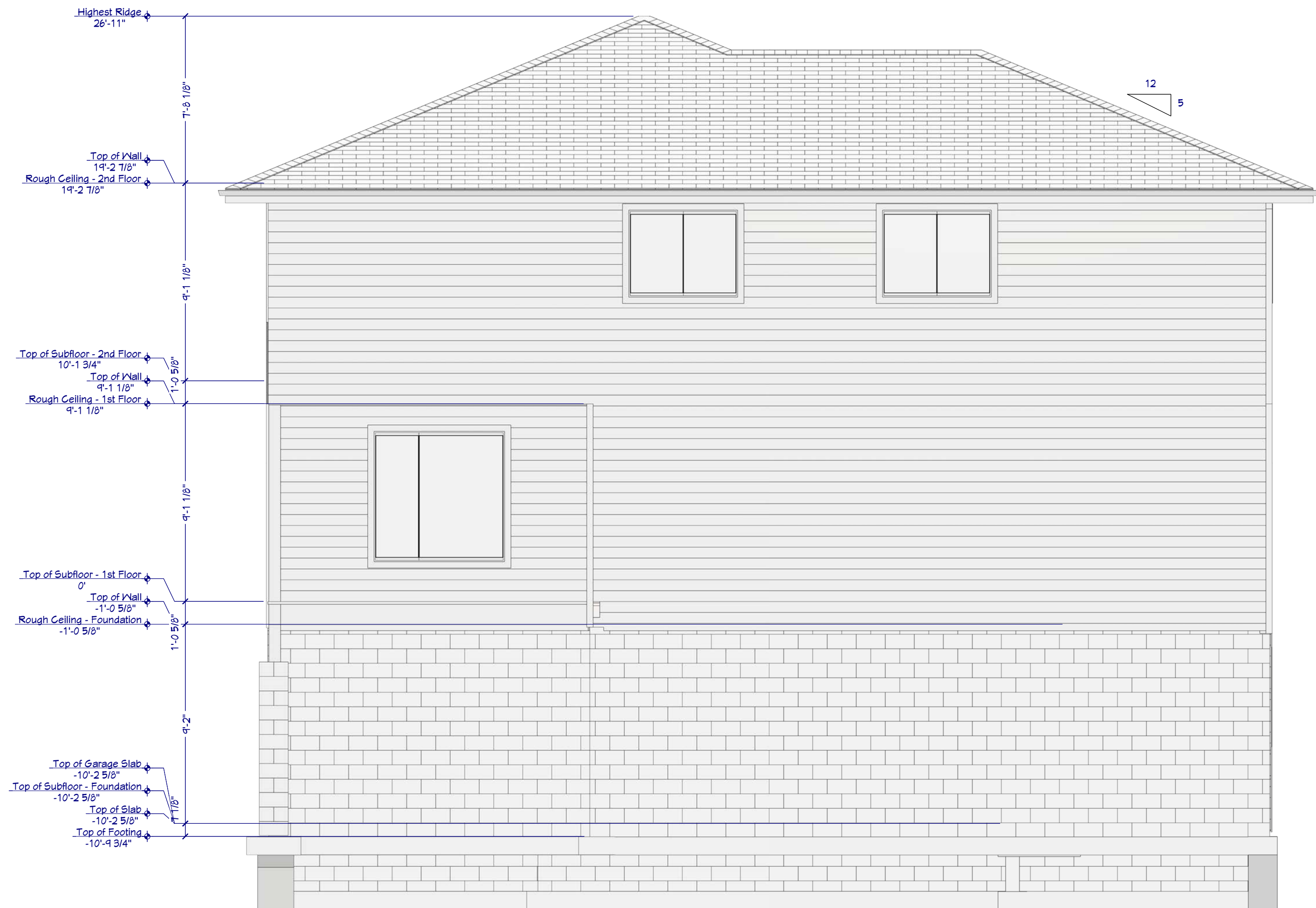
Exterior Elevation Back
